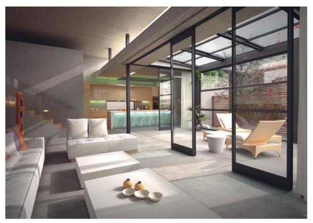
Convenient and automatic, simply press a button, glass panels can be moved to a variety of individually pre-programmed positions under fully automatic control. The integrated monitoring system ensured that stops the panel movement the moment contact is made with an obstacle. The system operating behavior can be easily adjusted by parameter reconfiguration.
